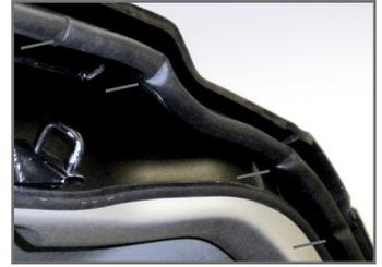
*Problem: Standard extruded seal kinks when following extreme curvature to maintain section.*
