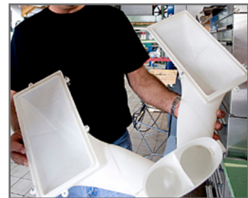
Prototype airbox printed in ABS.
