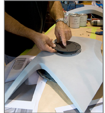
Gas cap inserted into printed rear fender section.
