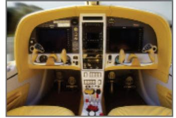
The dashboard cover was built on a Fortus 900mc, finished, and then installed directly in to the VUT100.
