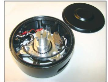
*The FDM enclosures are loaded with electrical, mechanical, and optical components.*
