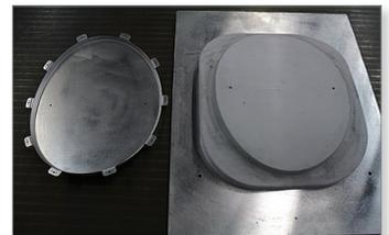
Aluminum window pan (left) and FDM tool
