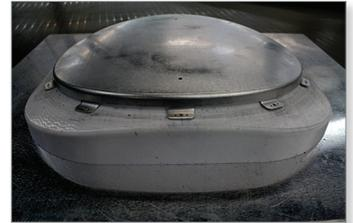
Aluminum window pan shown on top of FDM tool
